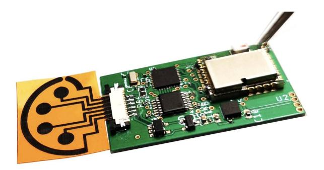
When attached to supporting electronics, the sensor can wirelessly transmit data to the user's cell phone through Bluetooth. Credit: Caltech
