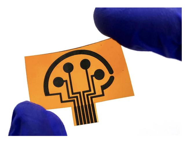
The sensor element is created from thin plastic etched with a laser. Credit: Caltech
