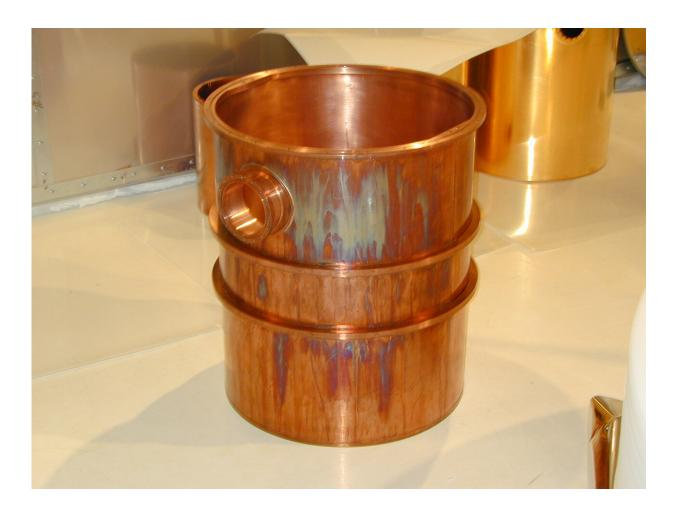
The SNOBOX — the device designed to detect dark matter particles for the SuperCDMS experiment — will use nesting copper cans similar to this one, which was used in the progenitor CDMS experiment at Soudan. Credit: Dan Bauer, Fermilab
