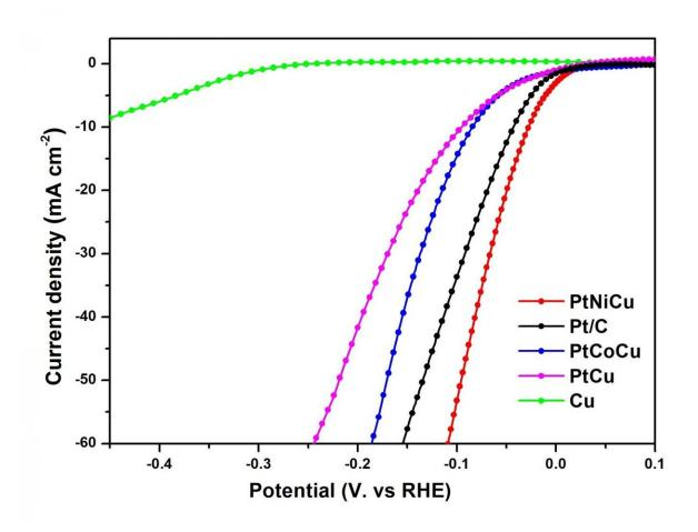
The HER polarization curves of hollow PtNiCu nanoparticles, commercial Pt/C, hollow PtCoCu nanoparticles, hollow PtCu nanoparticles and Cu nanoparticles in 1.0 M KOH aqueous solution at a scan rate of 5 mV s-1. Credit: Science China Press
