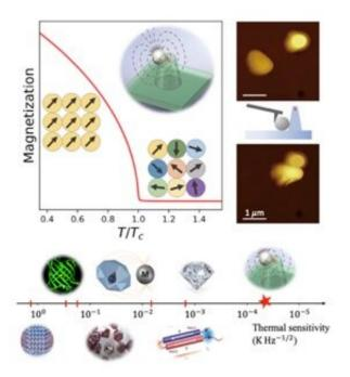
Upper left is the design of a hybrid nanothermometer composed of a single magnetic copper-nickel alloy nanoparticle and a single nitrogen-vacancy center in a diamond nanopillar. Upper right shows the nanomanipulation process with an atomic force microscope. Lower gives the sensitivity of different nanothermometers working under ambient conditions. Credit: @Science China Press
