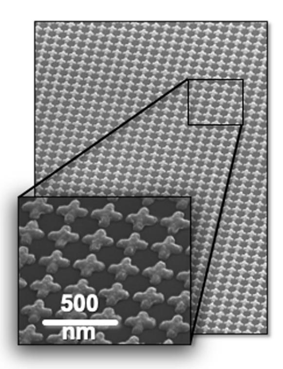
A scanning electron microscope image of the nanopatterned plasmonic metasurface that engineers from Rice University, the Polytechnic University of Milan and the Italian Institute of Technology created to modulate polarized light
