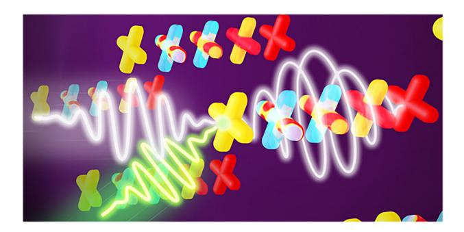
A pictorial schematic depicts the structure and action of a nanopatterned plasmonic metasurface that modulates polarized light at terahertz frequencies. An ultrashort laser pulse (green) excites cross-shaped plasmonic structures, which rotate the polarity of a second light pulse (white) that arrives less one picosecond after the first. Credit: A. Assié
