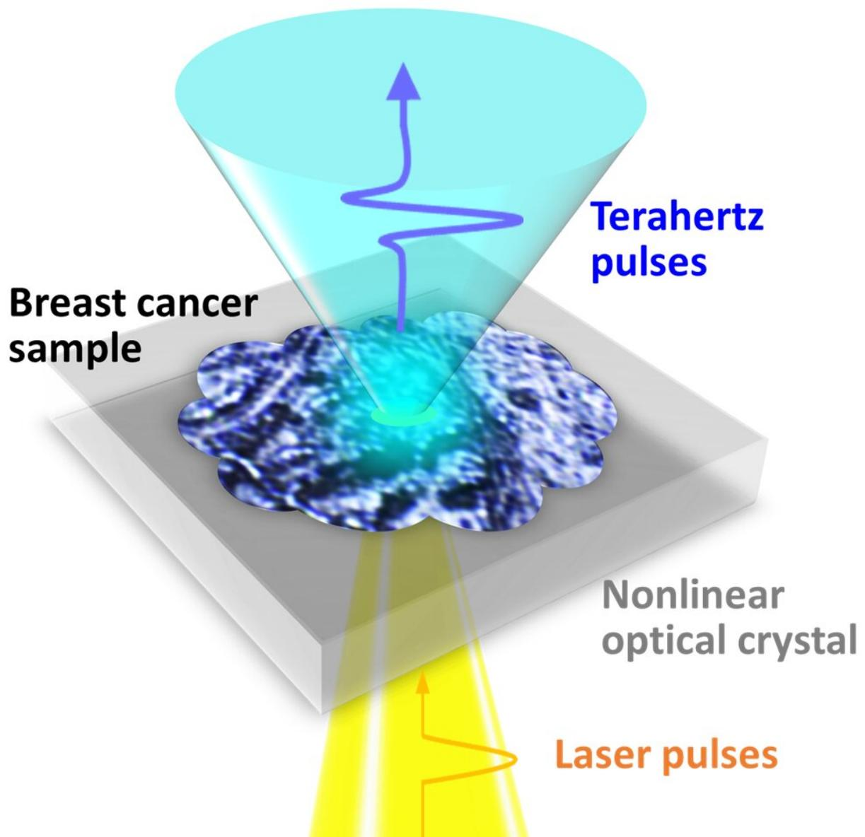
A schematic drawing of the measurement of breast cancer tissue fabricated on a nonlinear optical crystal. Credit: Osaka University
