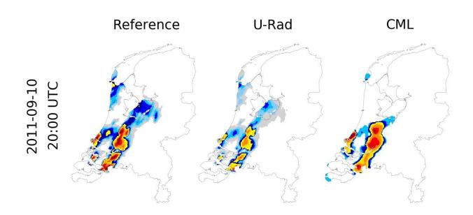
A comparison of estimated rainfall intensity in the Netherlands on 10-09-2011 22.00 hr. The reference (radar image corrected with KNMI precipitation data), the operational radar image (U-Rad) and the precipitation intensity as estimated using CML data. Credit: Wageningen University & Research
