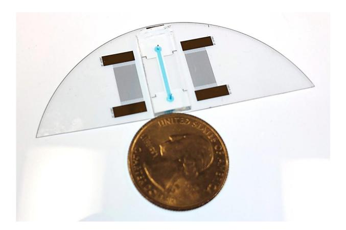
An Acousto Thermal Shift Assay "lab-on-a-chip" device shown next to a quarter for size comparison. Credit: CU Boulder College of Engineering and Applied Science
