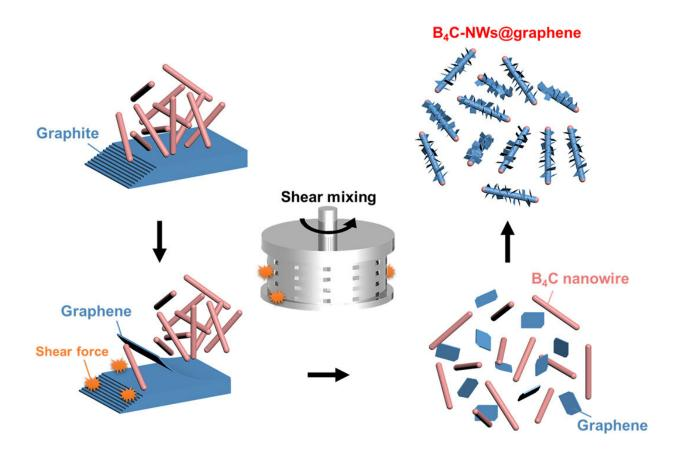
Schematic illustration of the synthesis process steps of B4C-NWs@graphene formation. Credit: Science Advances, doi: 10.1126/sciadv.aba7016
