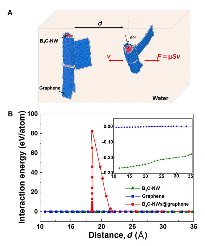
The MD simulations of the nanofiller interactions. (A) MD snapshots of the initial structure (B4C-NWs@graphene/B4C-NWs@graphene) for calculating the interaction energy. (B) Interaction energy profiles between two nanofillers of the
