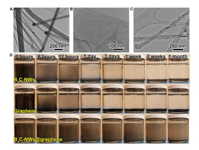
Synthesis of nanofillers in dilute water by shear mixing. TEM images of (A) B4C-NWs, (B) multilayered graphene, and (C) B4C-NWs@graphene. (D) Chronological digital photos of the suspensions of B4C-NWs, graphene, and B4C-NWs@graphene. Photo credit: Ningning Song, University of Virginia. Credit: Science Advances, doi: 10.1126/sciadv.aba7016
