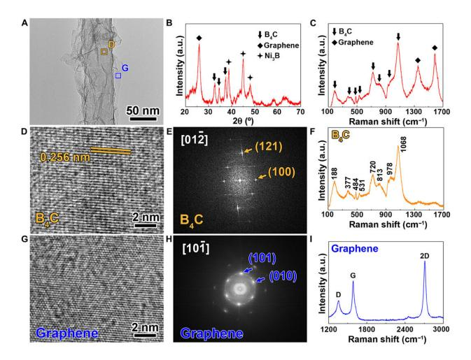
Characterization of B4C-NWs@graphene. (A) TEM image, (B) XRD pattern, and (C) background-corrected Raman spectrum of B4C-NWs@graphene. (D) HRTEM image, (E) the corresponding FFT, and (F) background-corrected Raman spectrum of the B4C-NWs in B4C-NWs@graphene. (G) HRTEM image, (H) the corresponding FFT, and (I) background-corrected Raman spectrum of the monolayered graphene in B4C-NWs@graphene. a.u., arbitrary units. Credit: Science Advances, doi: 10.1126/sciadv.aba7016
