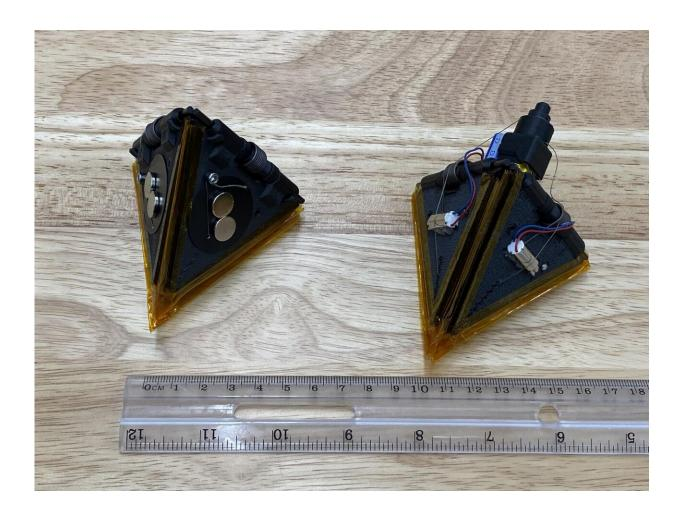
SwRI has designed a new technology to magnetically attach to metallic asteroids and sample their surfaces. Two Clockwork Starfish devices were tested in low gravity aboard Blue Origin's New Shepard rocket. Credit: SwRI
