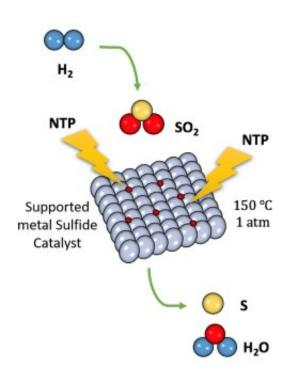
Schematic illustration of the plasma catalytic sulfur dioxide reduction with hydrogen or methane to sulfur at low temperature. Credit: Penn State
