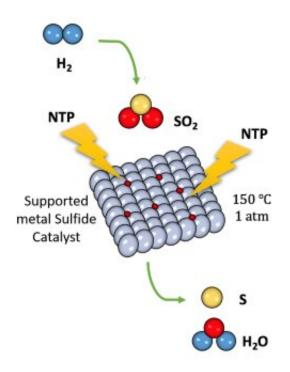
Schematic illustration of the plasma catalytic sulfur dioxide reduction with hydrogen or methane to sulfur at low temperature. Credit: Penn State
