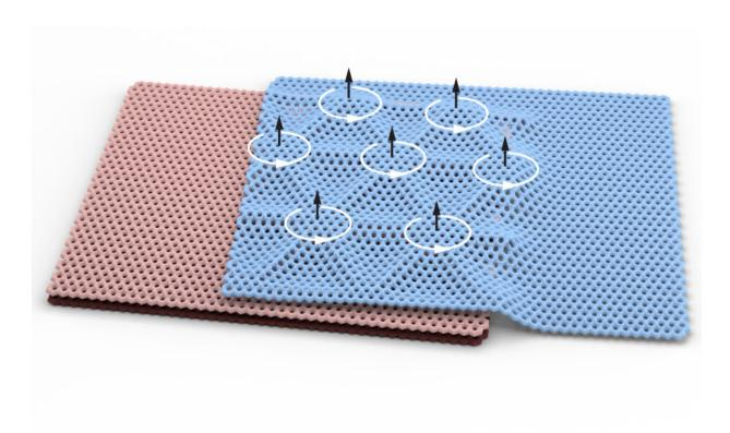
Stacking monolayer and bilayer graphene sheets with a twist leads to new collective electronic states, including a rare form of magnetism. Credit: Columbia University
