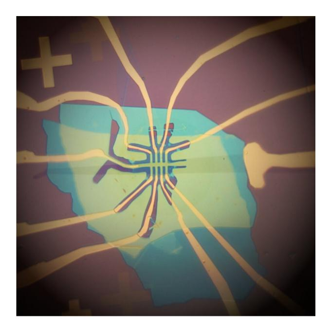
Optical microscope image of a twisted double bilayer graphene device. Credit: He et al.
