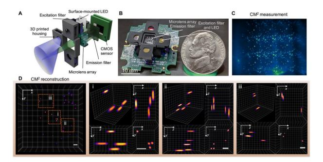
Single-shot 3D fluorescence CM2. (A) The CM2 combines an MLA optics and light-emitting diode (LED) array excitation in a compact and lightweight platform. (B) Picture of the CM2 prototype (the electric wires and the sensor driver are omitted). Photo credit: Yujia Xue, Boston University. (C) CM2 measurement on 100-µm fluorescent particles suspended in clear resin. (D) Projected view of the CM2 reconstructed volume (7.0 mm by 7.3 mm by 2.5
