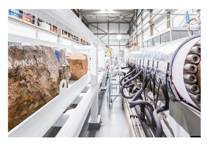
Downhole testing: match.BOGS simulates reservoir conditions down to several thousand meters. Credit: Fraunhofer-Gesellschaft
