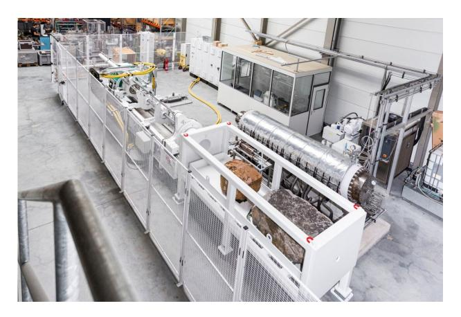
Fraunhofer IEG test rig enables the fast and economic examination of rock behavior under very extreme conditions. Credit: Fraunhofer-Gesellschaft
