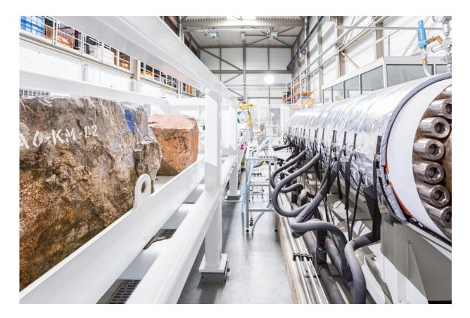
Downhole testing: match.BOGS simulates reservoir conditions down to several thousand meters. Credit: Fraunhofer-Gesellschaft
