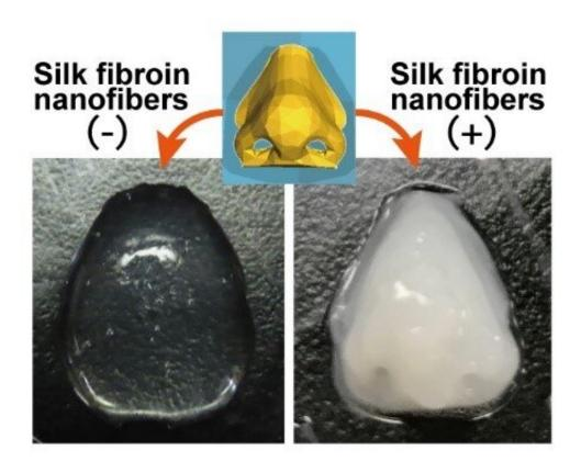
Figure. 3D printed constructs using hyaluronic acid-based inks free of silk fibroin nanofibers (-) and containing silk fibroin nanofibers (+). Credit: Osaka University
