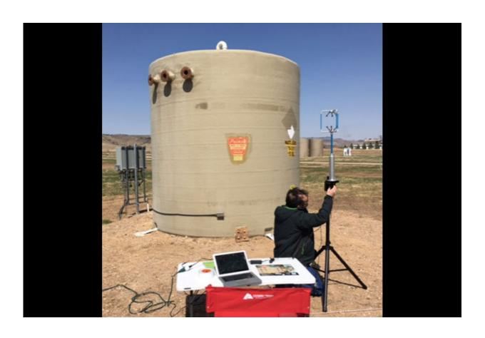
ALFaLDS is deployed during blind tests at the model oil and gas test facility at Fort Collins, Colorado. Credit: Los Alamos National Laboratory
