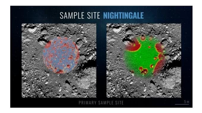
The OSIRIS-REx spacecraft will rely on this map to avoid hazards and touch down in an area where suitable sampling material is abundant. Green areas are safe for touch-down, while approaching red areas will cause the spacecraft to back away. The most promising areas for sample collection are marked purple. Credit: NASA/Goddard/University of Arizona
