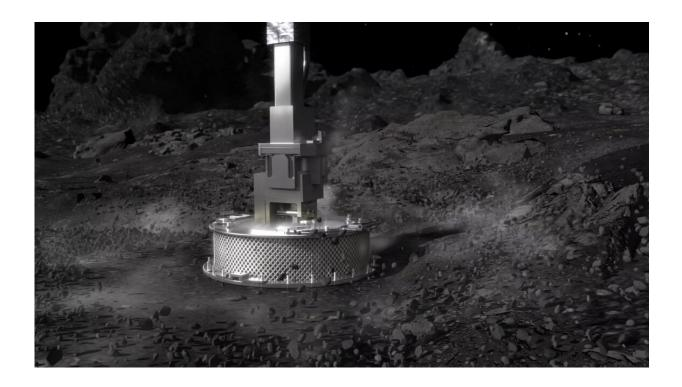
The sampler head of the OSIRIS-REx spacecraft works not unlike a reverse vacuum cleaner, designed to collect loose material from the surface of asteroid Bennu on Oct. 20. Credit: .NASA/Goddard Space Flight Center
