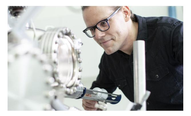
Lead author Ludwik Kranz with a scanning tunnelling microscope used to precisely place and encapsulate phosphorus atoms in silicon Credit: CQC2T
