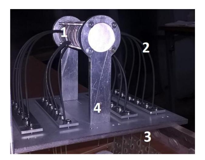
Device prototype: (1) the body of the detector consisting of scintillation disks, (2) fiber optics in a protective coating, (3) control boards for managing offset voltage and data acquisition, (4) prototype frame and stand for ground-based observations. Credit: Egor Stadnichuk et al./Journal of Instrumentation
