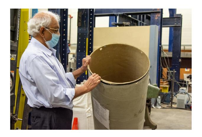
Hota GangaRao, Maurice A. and JoAnn Wadsworth Department of Civil and Environmental Engineering and director of the Constructed Facilities Center, in a lab. The newly innovated composite material made up of glass and polymer, will consist of a layer of high-density polyurethane foam to improve fatigue, puncture, and fire resistance of rail tank cars transporting hazardous materials. Credit: Paige Nesbit/WVU
