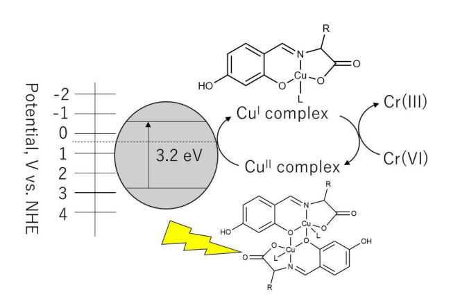
Chromium contamination in wastewater can be mitigated by converting Cr(VI) to Cr(III) through a photochemical reaction involving copper complexes. Credit: Takashiro Akitsu, Tokyo University of Science
