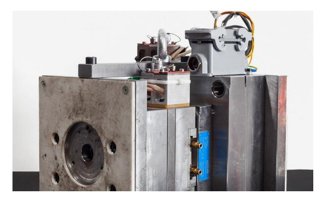
The Fraunhofer IPK team developed this injection molding tool to replicate prototype components made of polyhydroxybutyrate. Credit: Fraunhofer-Gesellschaft
