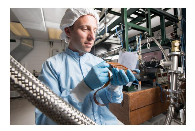
Fermilab scientist Javier Tiffenberg examines a skipper CCD in a cleanroom at Fermilab's Silicon Detector Facility. Credit: Reidar Hahn, Fermilab
