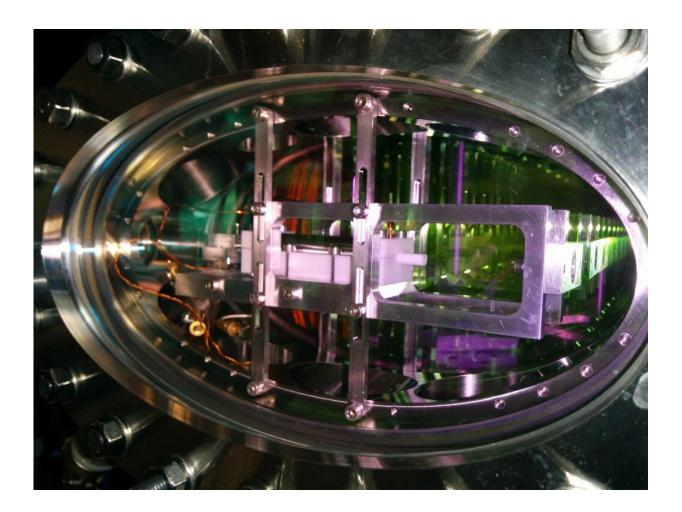
For the experiment, atoms of rubidium-87 are first pre-cooled and then transported to the main test area, which is a custom-made vacuum chamber. There they are cooled to temperatures of just a few microkelvins. Credit: Windpassinger group
