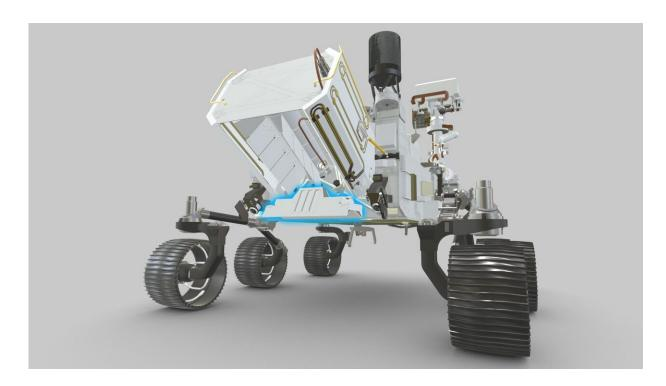
Perseverance's Radar Imager for Mars' Subsurface Experiment (RIMFAX) uses radar waves to probe the ground, revealing the unexplored world that lies beneath the Martian surface. Highlighted in blue in this visualization from the interactive tool Learn About Perseverance, the instrument's antenna is externally mounted underneath the Multi-Mission Radioisotope Thermoelectric Generator (MMRTG — the rover's nuclear battery) on the back of the Perseverance. Credit: NASA/JPL-Caltech
