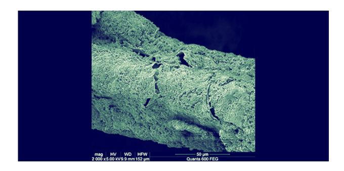
SEM image shows the dense and uniform cathodic biofilm, which mainly comprises chemolithoautotrophs, and could serve as biocatalysts for efficient carbon dioxide conversion to acetate. Credit: 2020 KAUST
