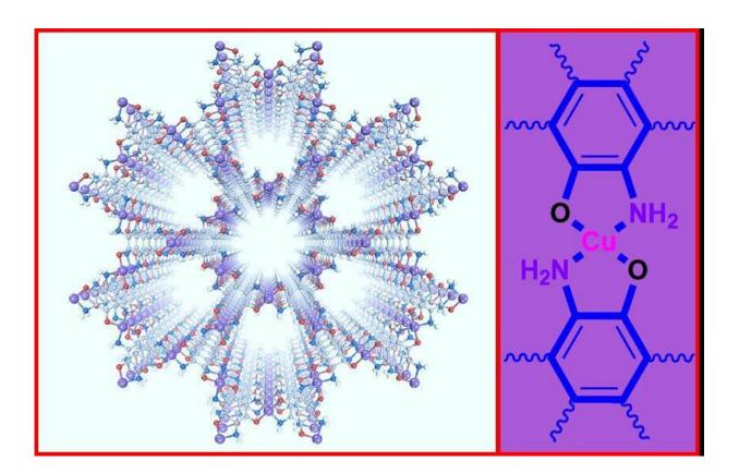
Figure 1.The structure of the Cu3(TABTO)2-MOF (carbon, nitrogen, oxygen, hydrogen, and copper atoms are gray, blue, red, white, and purple, respectively). Credit: Institute for Basic Science
