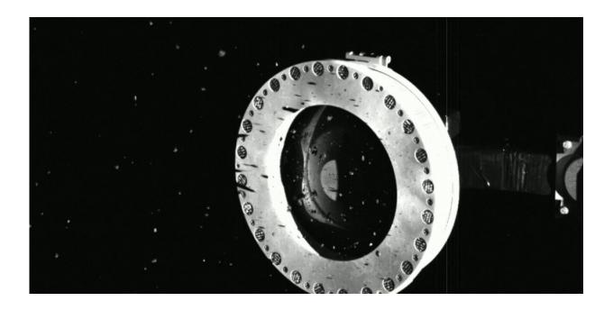
Captured by the spacecraft's SamCam camera on Oct. 22, 2020, this image shows that the sampler head on NASA's OSIRIS-REx spacecraft is full of rocks and dust collected from the surface of the asteroid Bennu. They show also that some of these particles are slowly escaping the sampler head through small gaps where the head's mylar flap is wedged open. Credit: NASA
