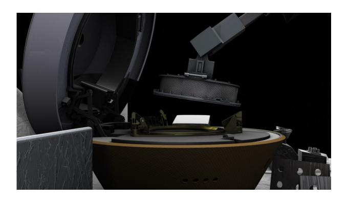
This illustration shows NASA's OSIRIS-REx spacecraft stowing the sample it collected from asteroid Bennu on Oct. 20, 2020. The spacecraft will use its Touch-And-Go Sample Acquisition Mechanism (TAGSAM) arm to place the TAGSAM collector head into the Sample Return Capsule (SRC). Credit: NASA/University of Arizona, Tucson
