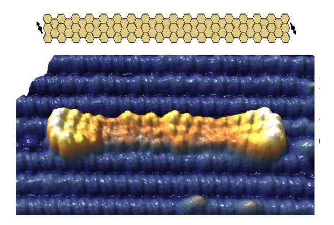
Scientists synthesized graphene nanoribbons, shown in yellow, on a titanium dioxide substrate, in blue. The lighter ends of the ribbon show magnetic states. The inset drawing shows how the ends have up and down spin, suitable for creating qubits. Credit: ORNL, U.S. Dept. of Energy
