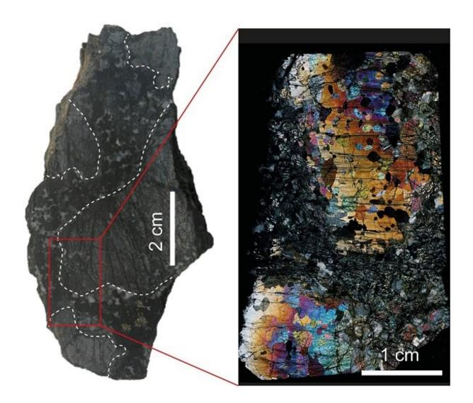
The fluid inclusions inside the olivine contain nanodiamonds, apart from serpentine, magnetite, metallic silicon and pure methane. Credit: University of Barcelona
