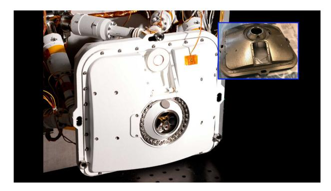
The outer shell of PIXL, one of the instruments aboard NASA's Perseverance Mars rover, includes several parts that were made of 3D-printed titanium. The inset shows the front half of the two-piece shell part it was finished. Credit: NASA/JPL-Caltech
