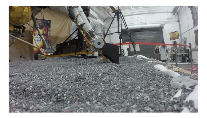
This footage from Aug. 19, 2019, shows a replica of InSight scraping soil with a scoop on the end of its robotic arm in a test lab at JPL. A replica of the "mole" - the lander's self-hammering heat probe - comes in to view as the scoop moves to the left. On Mars, InSight will scrape and tamp down soil on top of the mole to help it dig. Credit: NASA/JPL-Caltech
