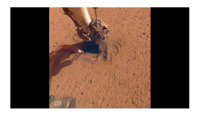
NASA's InSight retracted its robotic arm on Oct. 3, 2020, revealing where the spike-like "mole" is trying to burrow into Mars. The copper-colored ribbon attached to the mole has sensors to measure the planet's heat flow. In the coming months, the arm will scrape and tamp down soil on top of the mole to help it dig. Credit: NASA/JPL-Caltech
