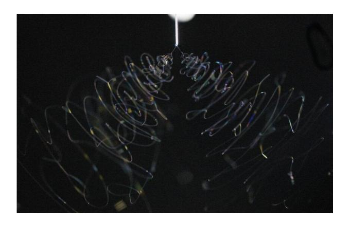
Liquid polymer is stretched out to create nanofibers used to increase the efficiency of cloth masks. Credit: BYU Photo
