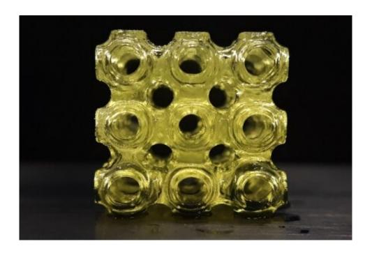
3-D-printed molecular ferroelectric metamaterial made of imidazolium perchlorate. Credit: University at Buffalo
