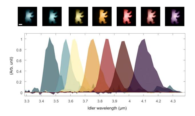
Multispectral imaging. Obtained signal transmission images for varying mid-IR illumination wavelengths. Scale bar, 2 mm. The spectra were recorded at the signal wavelength with a grating spectrometer and converted to the corresponding mid-IR wavelength. Credit: Science Advances, doi: 10.1126/sciadv.abd0264
