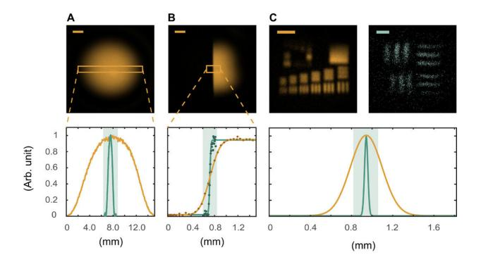
Characterization of the imaging arrangements. The images and data of the unmagnified and magnified setups are presented in orange and green, respectively. (A) Measured FoVs of the unmagnified and magnified setups are 9100 ± 82 and 819 ± 9  $\mu$ m, respectively. (B) Edge response functions fitted to the data of the two imaging arrangements. (C) Measured resolutions of the unmagnified and magnified setups are 322 ± 5 and 35 ± 5  $\mu$ m, respectively. The
