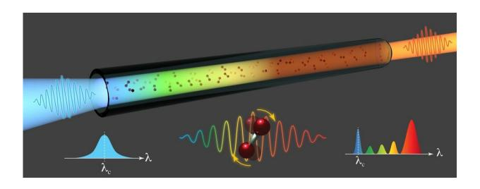
A laser optical pulse (blue) enters from the left into the hollow-core fibre filled with nitrogen gas (red molecules) and, along propagation, experiences a spectral broadening towards longer wavelengths, depicted as an orange output beam (right). This nonlinear phenomenon is caused by the Raman effect associated with the rotations of the gas molecules under the laser field, as schematically illustrated in the bottom panel. Credit: Riccardo Piccoli (INRS)
