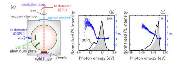
(a) A scheme of temperature variable ODPL spectroscopy. The spectra of ODPL and SPL as well as r (ODPL intensity divided by SPL intensity) measured at (b) T = 300 K and (c) T = 12 K. Credit: Kazunobu Kojima
