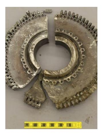
A NTSB photograph of a cracked metal disk from an airline engine caused by the type of metal fatigue that the new method would be able to predict long before a crack ever appears. Credit: NTSB
