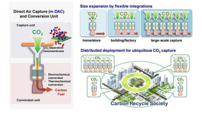
Technological solutions for the CO2 emission into the atmosphere should include variety of approaches as there is no one "silver bullet" solution. In this work researchers from I2CNER, Kyushu University and NanoMebrane Technologies Inc. Japan suggest using the gas separation membranes as a tool for direct air capture. When combined with advanced technologies for CO2 conversion the envisaged systems can be widely employed in carbon-recycling sustainable society. Credit: Kyushu University
