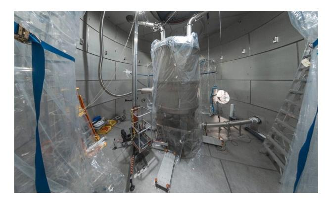
LZ's central detector, pictured here during assembly, is located inside a large water tank on the 4850 Level of Sanford Lab, nearly a mile underground. LZ will search for theorized dark matter particles known as WIMPs. Credit: Nick Hubbard/Sanford Lab
