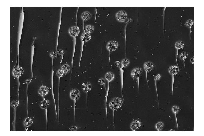
The micro-reservoirs of lipid vesicles in the bulk of the hydrogel, as seen by scanning electronmicroscopy when the gel is fractured at low temperatures to expose an inner surface. Credit: Lin et al., Science (2020)
