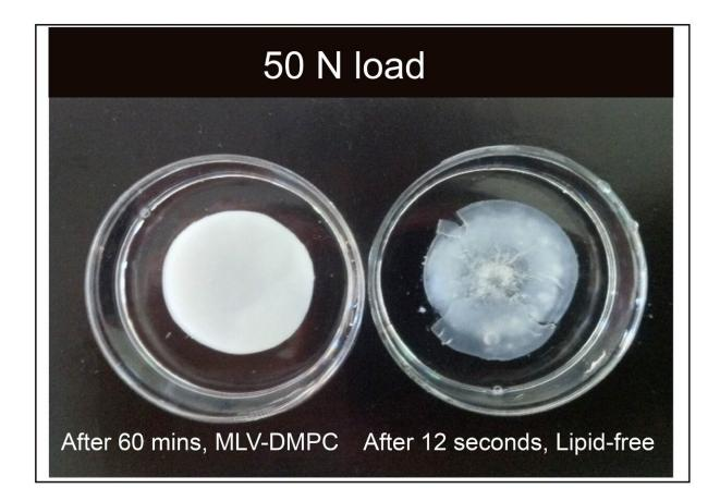
Shows one striking effect of the very efficient lubrication: hydrogel disks are compressed by a steel sphere under a 5 kg load, which is then rubbed back-andforth on them. When lipids are added to the gel to lubricate it, as in the picture on the left, then even after an hour's back-andforth sliding there is hardly any change to the gel because the friction is so low. Credit: Lin et al., Science (2020)
