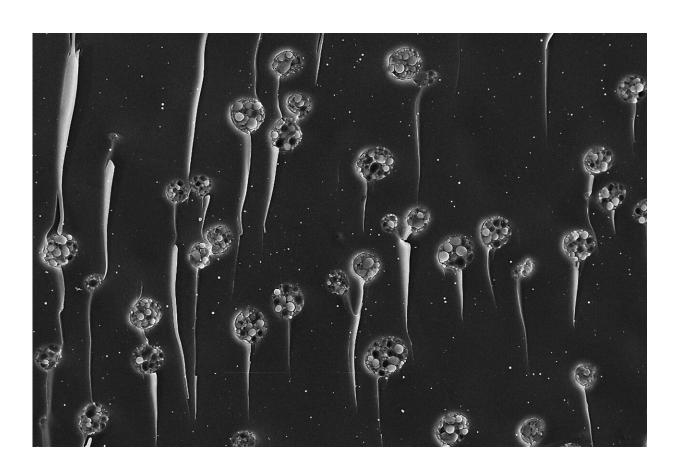
The micro-reservoirs of lipid vesicles in the bulk of the hydrogel, as seen by scanning electronmicroscopy when the gel is fractured at low temperatures to expose an inner surface. Credit: Lin et al., Science (2020)
