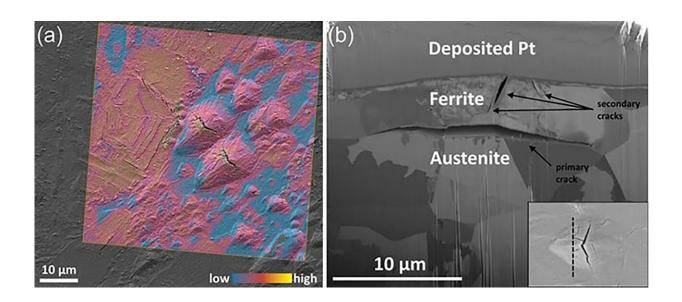
Hydrogen can cause brittleness in several metals including ferritic steel, but recent advancements provide insight into the embrittlement process.a) The arrowhead-shaped delaminations in stainless steel reveal cracks with significantly higher deuterium concentrations b) Secondary ion cross-sectional profile for one such delamination. Credit: O. Sobol, G. Holzlechner, G. Nolze, T. Wirth, D. Eliezer, T. Boellinghaus, and W.E.S. Unger
