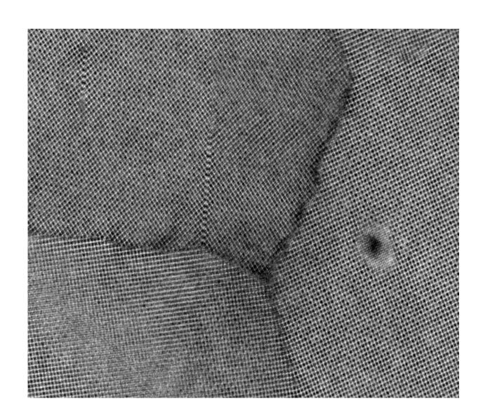
Image illustrates several of the phenomena that the team has been able to describe for the first time, including a range of grain boundaries, extended planar defects, stacking faults, and local inclusions of non-perovskite material. Credit:
