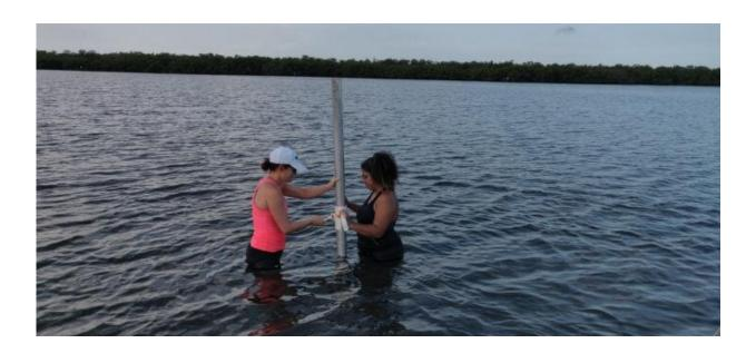
Dr. Joanne Muller (left) and Ilexxis Morales (right) using a hand coring technique, with a 3-meter core and core candles around the aluminum pipe, in Florida's Indian River Lagoon. Credit: James Javaruski.
