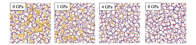
The voids in silica glass (yellow), which are responsible for scattering of light and degradation of signals, become much smaller when the glass is quenched at higher pressures (Yongjian Yang, et al., npj Computational Materials, September 17, 2020). Credit: Yongjian Yang, et al., npj Computational Materials, September 17, 2020
