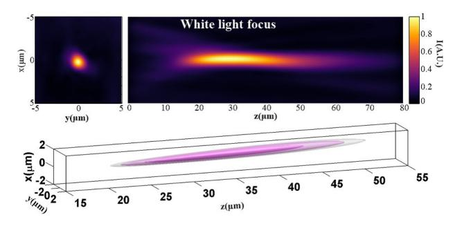
Photonic jet focused by a graphene oxide microbubble lens. Credit: H. Lin et al., doi 10.1117/1.AP.2.5.055001
