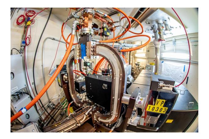
Over the course of two years, crews at SLAC installed a state-of-the-art high brightness electron source and new electron bunch compressor systems for producing intense beams. They also upgraded the facility's control systems and installed tools to analyze the beam properties. Credit: Jacqueline Orrell/SLAC National Accelerator Laboratory
