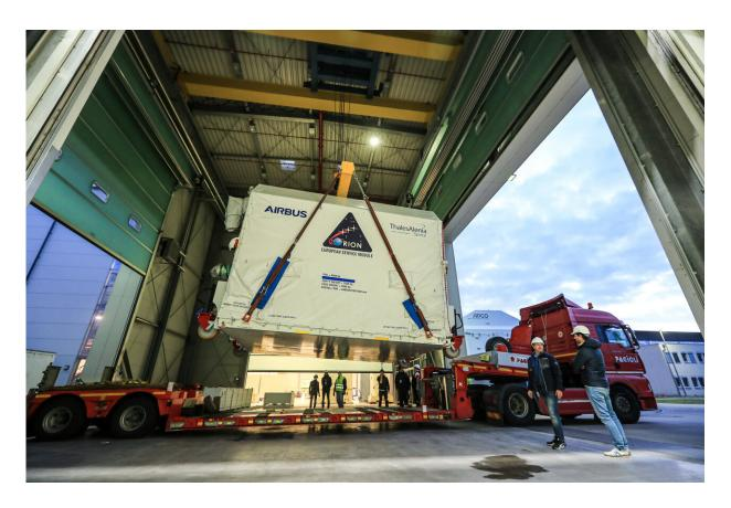
The structure that will fly the first woman and next man to land on the Moon and return on the Artemis III mission by 2024 arrives at the Airbus integration hall in Bremen, Germany, from its Thales Alenia Space manufacturing site in Turin, Italy. The structure was transported in an oversized container that keeps the temperature and humidity levels constant, taking a week to travel the 1200 km trip. Credit: Airbus
